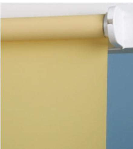
**Features:** White plastic brackets with 25 or 38mm aluminium barrel and strong, constant tension spring mechanism. Aluminium bottom bar, fabric covered at front. Pull-cord with cleat, and pulleys for single or double-corded operation.
