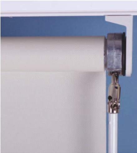
**Features:** Heavy-duty white plastic covered / metal brackets for face or top fixing, with 53/60mm grooved aluminium barrel. Fabric is located in the groove in such a way that, although it cannot be pulled out it may be slid out sideways for repair or replacement. A compact but very strong gear control is bolted to one of the brackets and is operated by a fixed crank handle. The rigid white plastic bottom bar is fabric covered at front.
