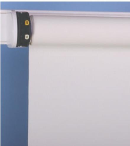
**Features:** Heavy-duty white plastic covered / metal brackets for face or top fixing, with 53/60mm grooved aluminium barrel. Fabric is located in the groove in such a way that, although it cannot be pulled out it may be slid out sideways for repair or replacement. A powerful 240v AC motor is housed within the barrel and is operated by an individual switch. The rigid white plastic bottom bar is fabric covered at front.
