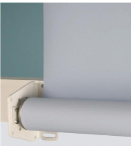
**Features:** Twin barrel system with white aluminium brackets. Fabric mounted on sprung 57mm aluminium barrel. Aluminium bottom bar, fabric covered at front, attached to two draw tapes. These tapes are attached, between flanged guides, to the 53mm drive barrel, operated by gear control and crank handle (R56) or 240v AC electric motor (R57).
