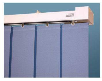
Features: 45 x 36.5mm white aluminium headrail with top-fix brackets and wheeled carrier trucks. The constant transport of the lourres is guaranteed by a precise aluminium spindle shaft. Electric 240V operation with built in slip dutch for both lourre tilt and draw. 127 mm/89mm lourres with weights and white stabilising chain. Single or split draw.
