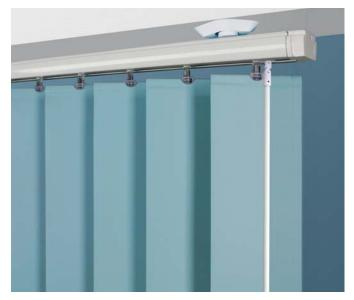
Kestrel: The KVL31 is specially adapted using the Kestrel Magnetic Anti-Ligature System so as to make it suitable for use in areas of self harm and mental health. Features: 40 x 25mm premium profiled white aluminium headrail with top-fix brackets and wheeled replaceable truck hooks.
